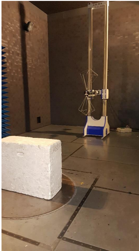
Radiated measurement setup between 200 MHz to 1000 MHz
