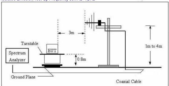
(C) Radiated Emission Test-Up Frequency Above 1GHz
