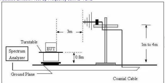
(C) Radiated Emission Test-Up Frequency Above 1GHz
