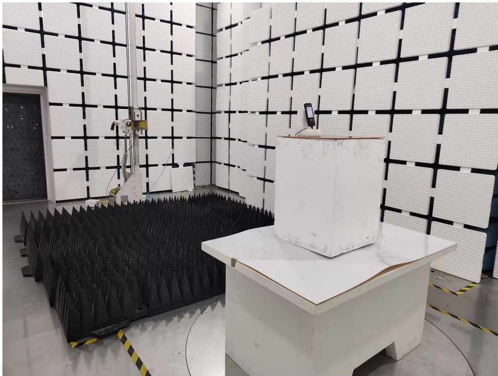
Radiated Emissions Measurement (Above 1GHz)
