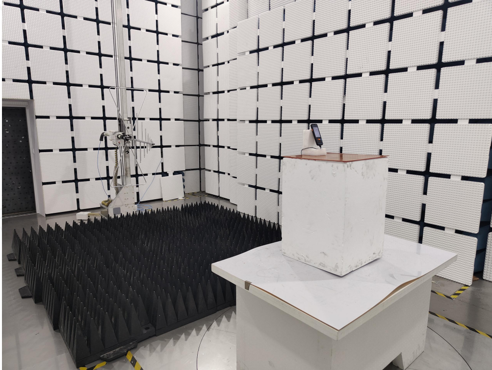
Radiated Emissions Measurement (Below 1GHz)
