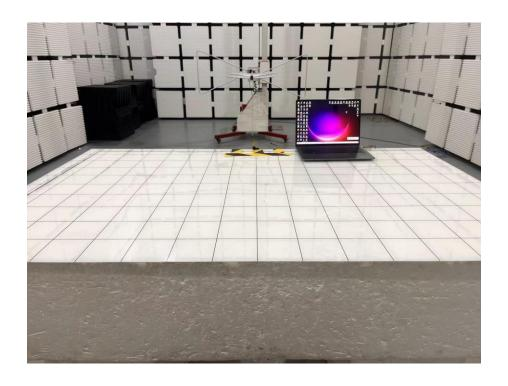
Set-up for Radiated Spurious Emission, Above 1GHz
