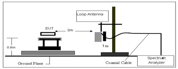
(B) Radiated Emission Test-Up Frequency 30MHz~1GHz
