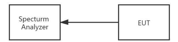
The EUT which is powered by the \${ POWER BY}, is connected to the Spectrum Analyzer; the RF load attached to the EUT antenna terminal is 50 Ohm; the path loss as the factor is calibrated to correct the reading. Make the measurement with the spectrum analyzer's resolution bandwidth(RBW) = 100 kHz. In order to make an accurate measurement, set the span greater than RBW.
