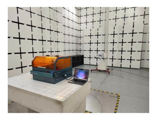
**Set-up for Radiated Spurious Emission, Above 1GHz**
