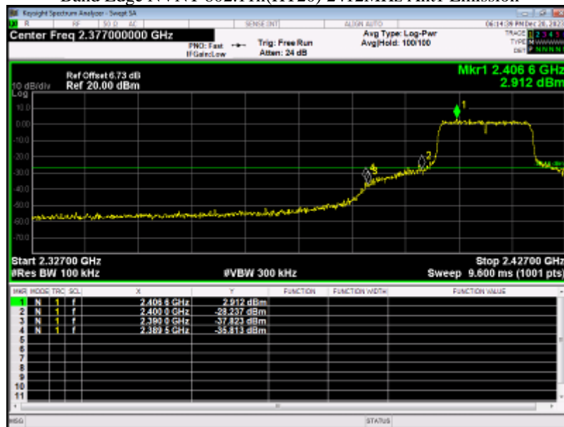
Band Edge NVNT 802.11n(HT20) 2412MHz Ant1 Emission
