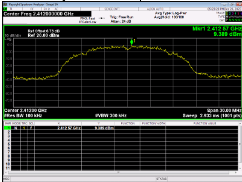
Band Edge NVNT 802.11b 1Mbps 2412MHz Ant1 Emission
