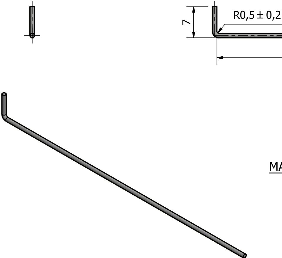
MATERIAL :  $\varnothing$  1 mm COPPER + TIN PLATING
