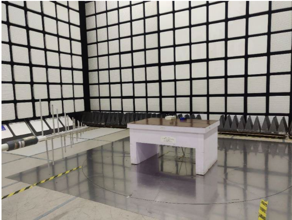
Figure 13: Photograph of RE test setup from 200MHz to 1GHz_Vertical polarization
