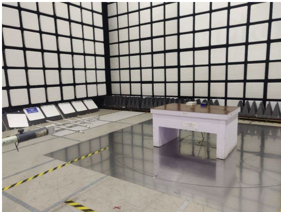
Figure 12: Photograph of RE test setup from 200MHz to 1GHz_Horizontal polarization
