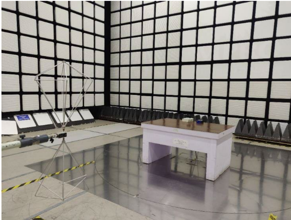
Figure 11: Photograph of RE test setup from 30MHz to 200MHz_Vertical polarization
