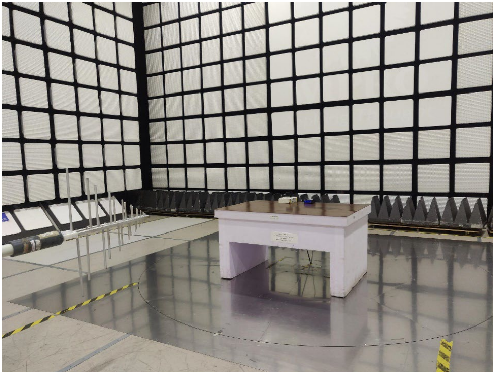
Figure 4: Photograph of RE test setup from 200MHz to 1GHz_ Vertical polarization
