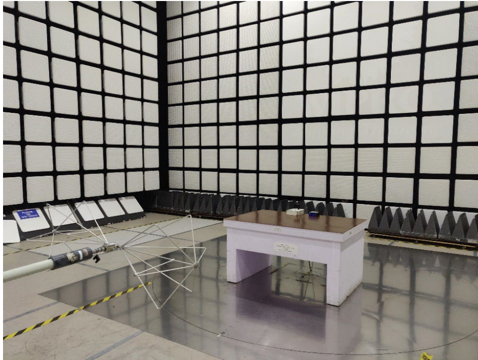
Figure 1: Photograph of RE test setup from 30MHz to 200MHz_ Horizontal polarization
