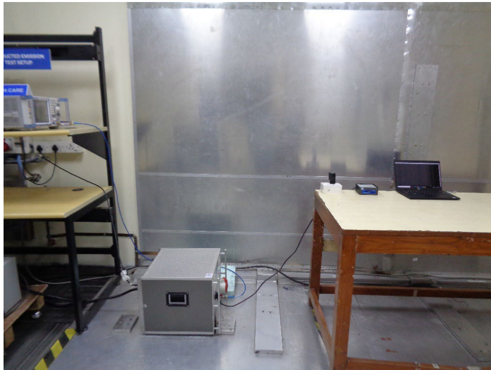
Figure 7: Photograph of CE test setup on Power port
