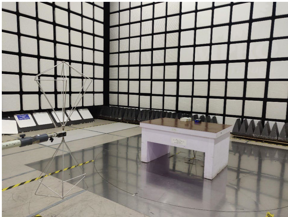
Figure 2: Photograph of RE test setup from 30MHz to 200MHz_ Vertical polarization
