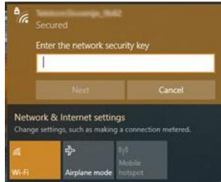
3. Use the **Security Key** printed on the label on the bottom part of the Home Gateway to connect to the Network.
