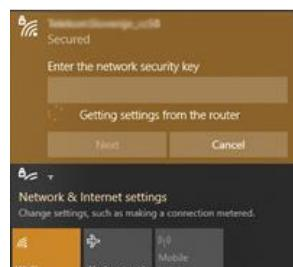
3. Press and hold WPS button on the back side of the Home Gateway for 1-3s. 2.4G and 5G light indicators should start blinking;
