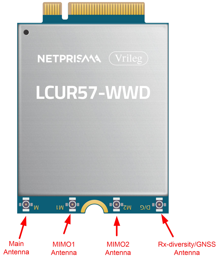
Figure 21: Antenna Connectors on the LCUR57-WWD Module
