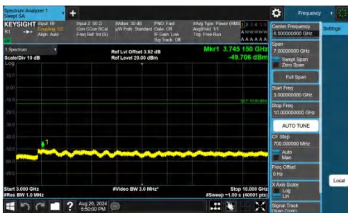
Band26(824-849)-3MHz-QPSK-26915-1RB#0-3000~10000-PASS
