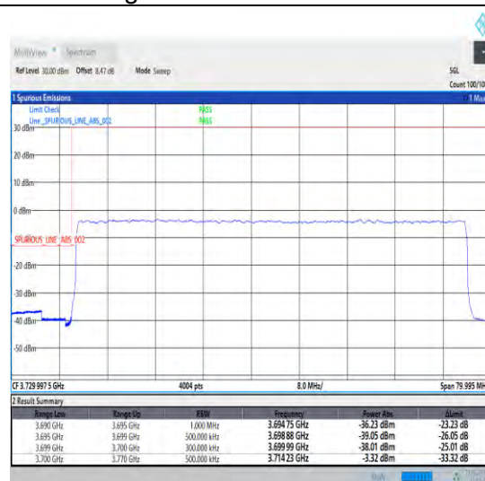
1-N77-3700-3980-30-70-L-3-DFT-PI2BPSK-Outer _Full-180@0-Ant0-1--PASS-see graph
