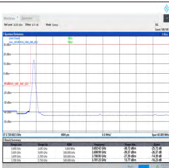
1-N77-3700-3980-30-50-L-1-DFT-PI2BPSK-Edge_1RB _Left-1@0-Ant0-1--PASS-see graph
