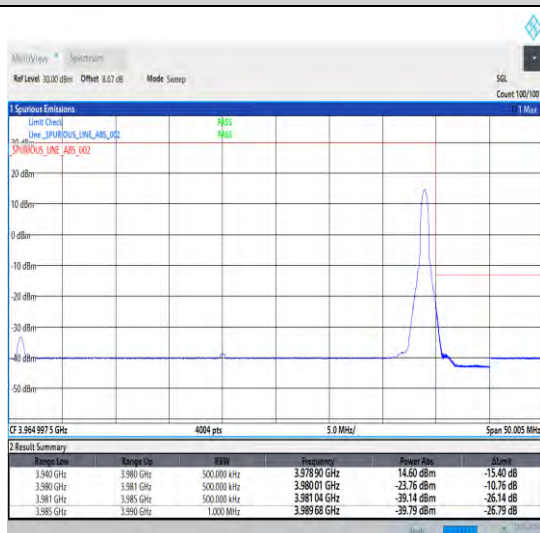
1-N77-3700-3980-30-40-H-5-CP-QPSK-Edge_1RB_Ri ght-1@105-Ant0-1--PASS-see graph
