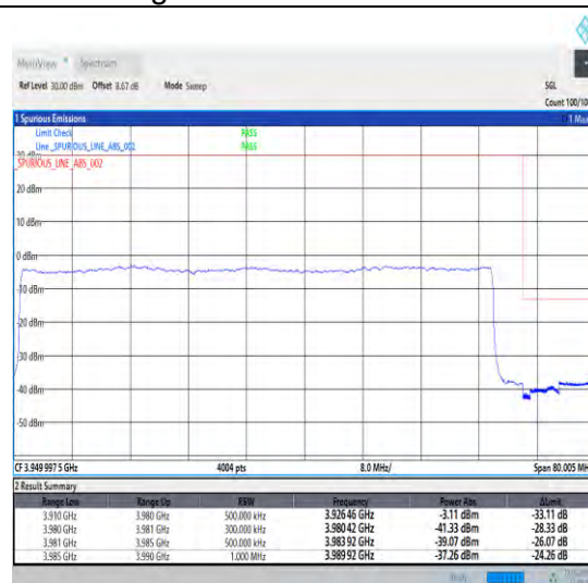
1-N77-3700-3980-30-70-H-3-DFT-PI2BPSK-Outer _Full-180@0-Ant0-1--PASS-see graph
