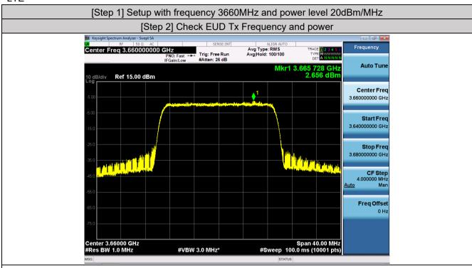
EIRP PSD=2.656-6.19+4.5=0.966dBm/MHz, Antenna gain is -6.1dBi, the path loss is 4.5dB, [Step 3] EUD stops transmission within 10 seconds of receiving instructions from its associated CBSD.
