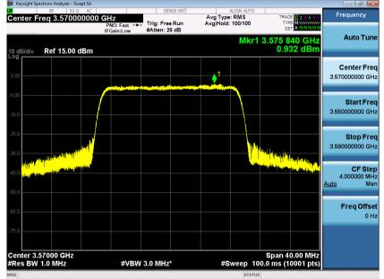
EIRP PSD=0.932-6.1+4.5=-1.068dBm/MHz, Antenna gain is -6.1dBi,the path loss is 4.5dB,
