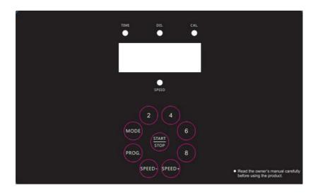
**TIME:** Displays your elapsed workout time in minutes and seconds. Time starts counting up from 5:00 to 99:00 per 1 second increment. You may also pre-set target time in STOP MODE-H1 before training.
