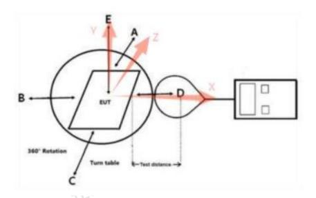
Note: The distance of the points A/B/C/D/E/F is 0,2,4,6,8,10,12,14,16,18, 20cm. The values tested by the probe are X, Y, and Z on three axes perpendicular to the edge of the device. Top and bottom side coincident with the axis(Y) of the main coil.
