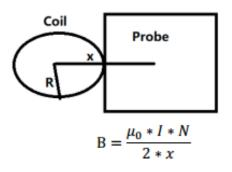
B(Unit:A/m): means H-field value;  $\mu_0$  is space permeability;  $\mu 0 = 4\pi \times 10^{-7}$ ;
