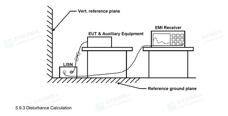
The AC mains conducted disturbance is calculated by adding the 10dB Pulse Limiter and Cable Factor and Duty Cycle Correction Factor (if any) from the measured reading. The basic equation with a sample calculation is as follows:
