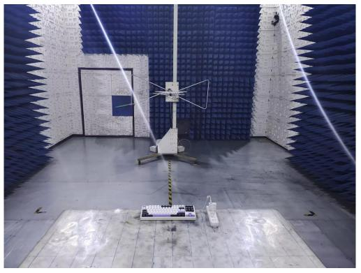
RADIATED EMISSION TEST SETUP ABOVE 1GHz
