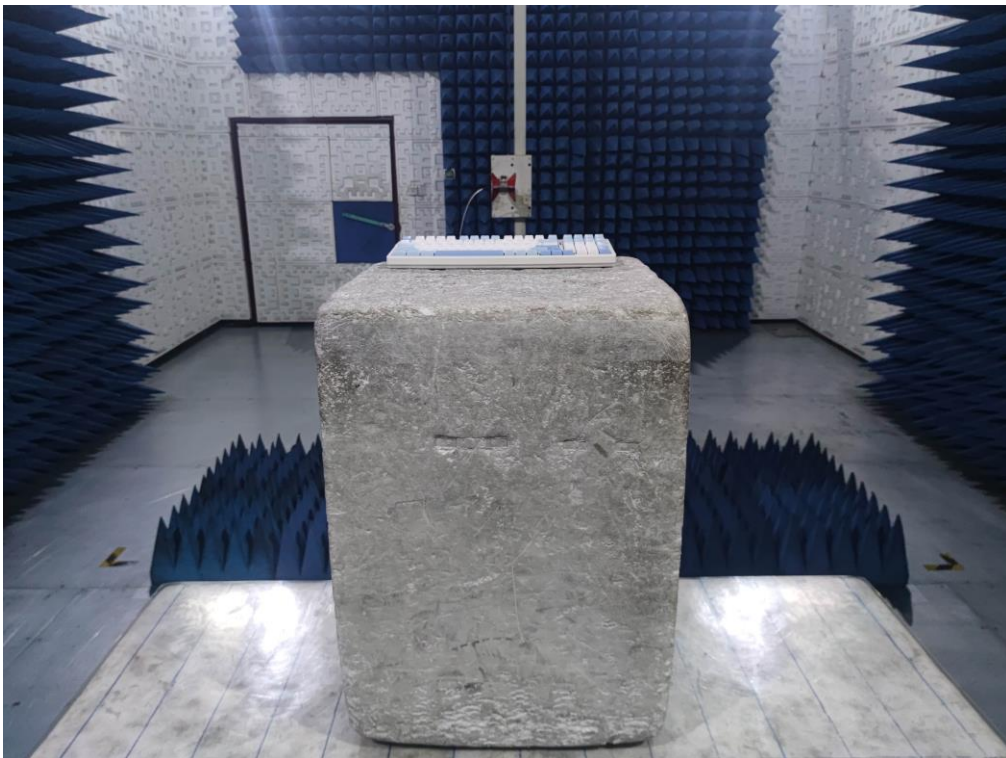
RADIATED EMISSION TEST SETUP ABOVE 1GHz
