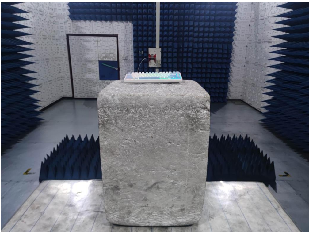
RADIATED EMISSION TEST SETUP ABOVE 1GHz
