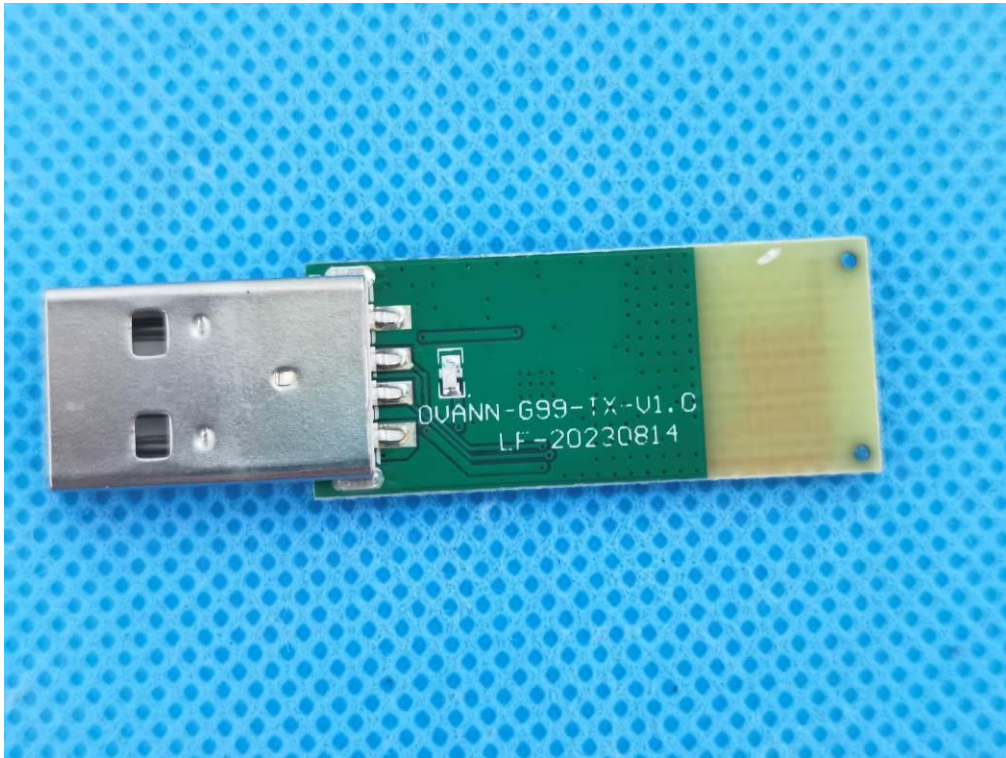
INTERNAL VIEW OF EUT (FIGURE 3)
