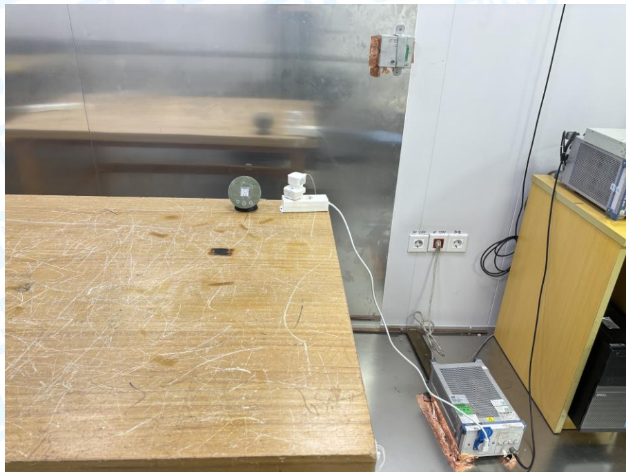
Photo of Setup for Conducted Emission
