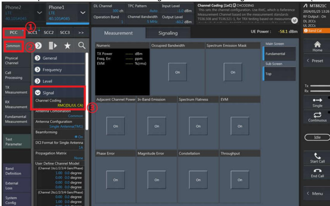
3. PCC parameter Settings: on the screen, and then select the PCC tab and Set operating band, BW, channel and RB configurations for PCC;
