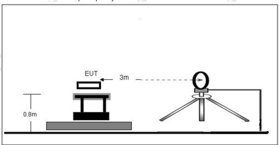
(B) Radiated Emission Test-Up Frequency 30MHz~1GHz
