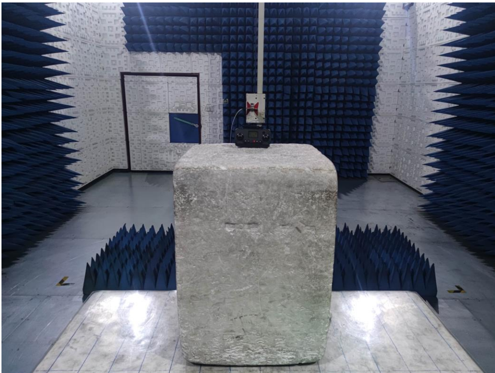
RADIATED EMISSION TEST SETUP ABOVE 1GHz
