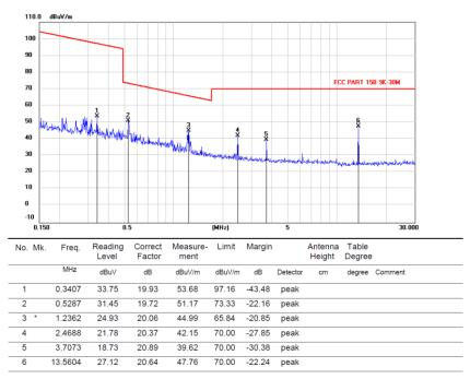
Note:1. \*:Maximum data; x:Over limit; I:over margin. 2.Measurement=Reading Level+Correct Factor; Correct Factor=Antenna Factor+Cable Loss.
