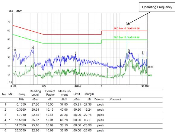
\*:Maximum data x:Over limit !:over margin Note: Measurement=Reading Level+Correc Factor. Factor=(LISN or ISN or PLC or Current Probe)Factor+Cable
