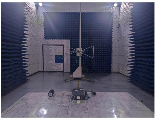
RADIATED EMISSION TEST SETUP BELOW 1GHz BY BATTRY
