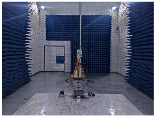
RADIATED EMISSION TEST SETUP-ABOVE 30MHz BY DC POWER
