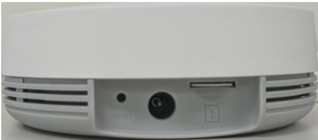
1. Insert the provided USIM into the Usim connector in the correct direction.
