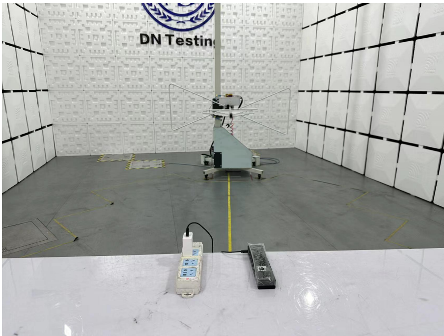
Radiated Emission Test View|(Below 1G)
