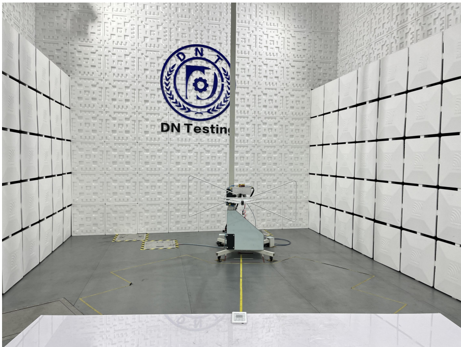
Radiated Emission Test View|(Below 1G)
