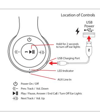
Charging the Headphones Insert the small connector of the supplied Type-C charging cable into the Type-C charging port on the headphones. Insert the large connector into a USB power source, such as the USB port on a computer, or into a 5V USB adapter (not included) and plug into a wall socket. The LED indicator will turn RED while charging, and will turn blue when fully charged.
