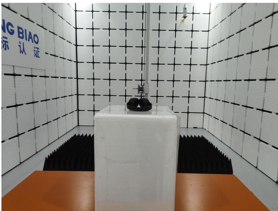
Radiated Emission Above 1GHz
