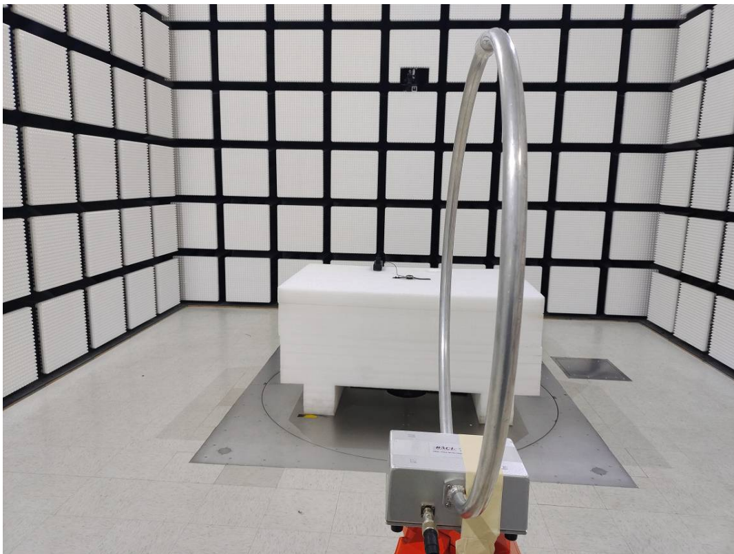
Radiated Emission Below 30MHz View Perpendicular
