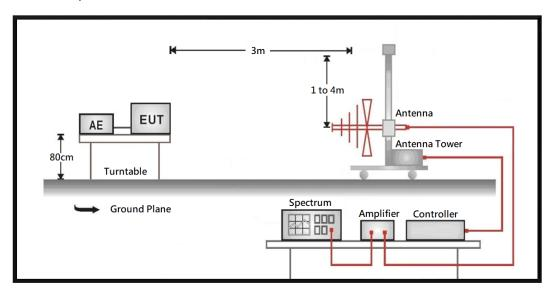
Radiated Spurious Measurement: above 1GHz
