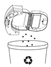
Remove the filter assembly and the high efficiency filter hipa can be washed or patted to remove dust. After washing, please dry before use.
