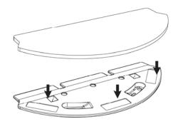
2 remove or install the water tank Disassembly: hold down the red dot on the back, pull back, take out the water tank. Installation: Push the water tank horizontally along the host card slot until you hear a "click";
