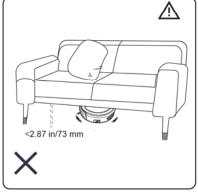
The robot cannot be used in a space lower than 73mm in height.
