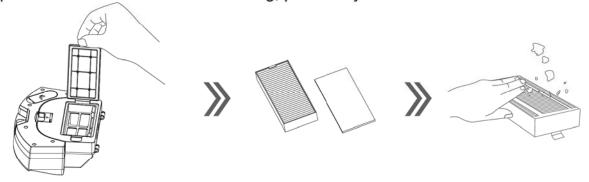
Wash the dust box and primary filter, air the dust box and filter assembly, and keep dry to engure their service life.
