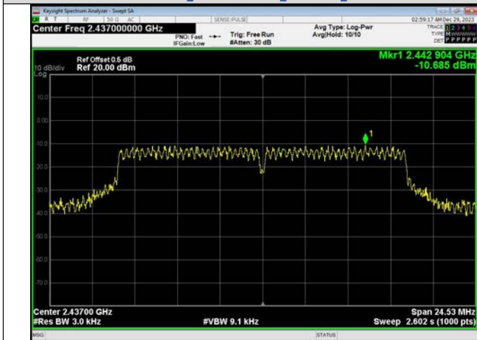
IEEE 802.11g_Channel 6_20MHz_Antenna 1
