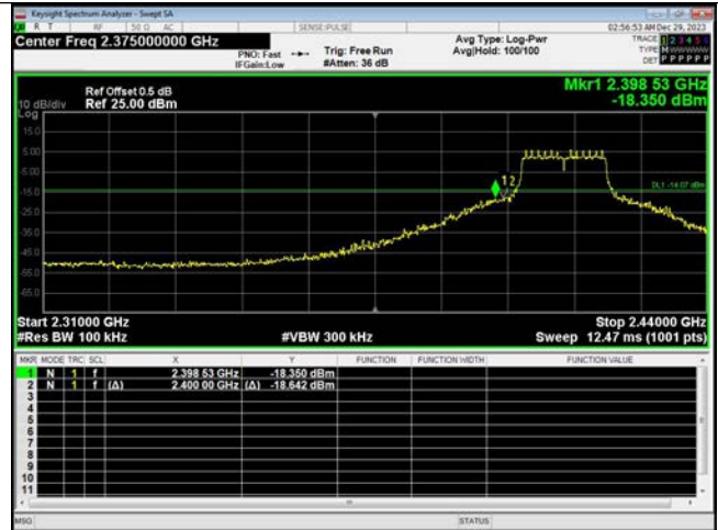
Out Of Band Emission IEEE 802.11g Channel 1_20MHz Antenna 1
