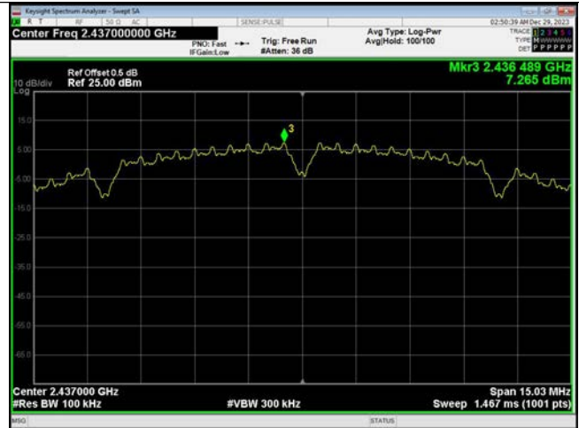
In-Band Reference Level IEEE 802.11b Channel 6_20MHz_Antenna 1
