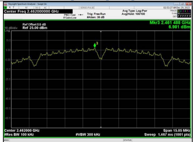
In-Band Reference Level IEEE 802.11b Channel 11_20MHz_Antenna 1
