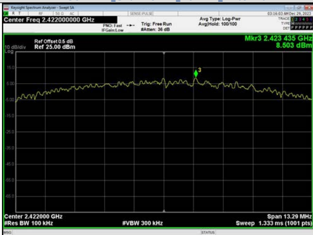
In-Band Reference Level IEEE 802.11n Channel 3 40MHz Antenna 1
