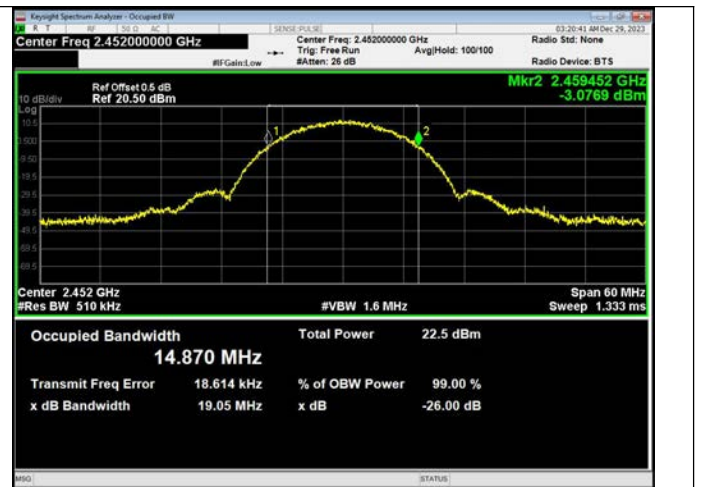
IEEE 802.11n_Channel 9_40MHz_Antenna 1
