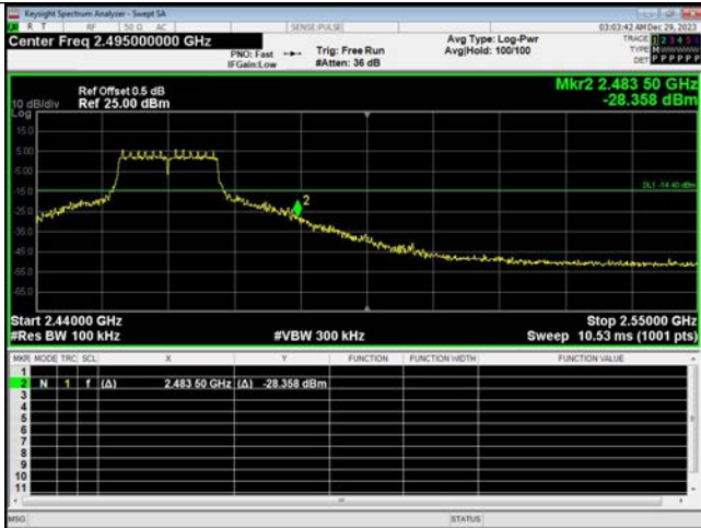
Out Of Band Emission IEEE 802.11g Channel 11_20MHz_Antenna 1
