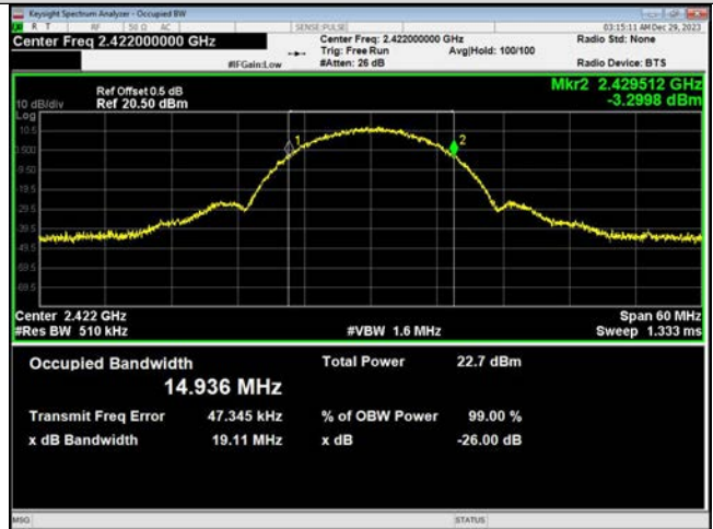
IEEE 802.11n_Channel 3_40MHz_Antenna 1
