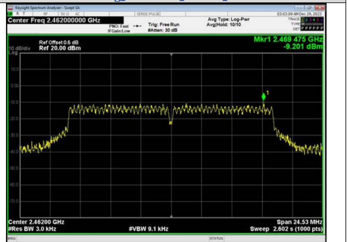
IEEE 802.11g_Channel 11_20MHz_Antenna 1
