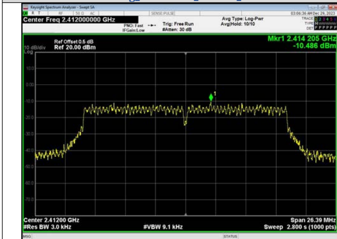
IEEE 802.11n_Channel 1_20MHz_Antenna 1
