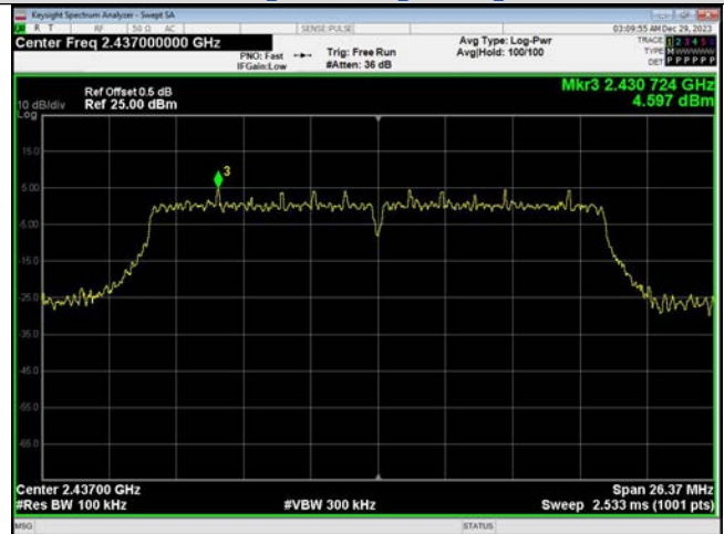
In-Band Reference Level IEEE 802.11n Channel 6_20MHz_Antenna 1
