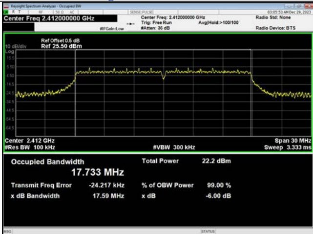
IEEE 802.11n_Channel 1_20MHz_Antenna 1
