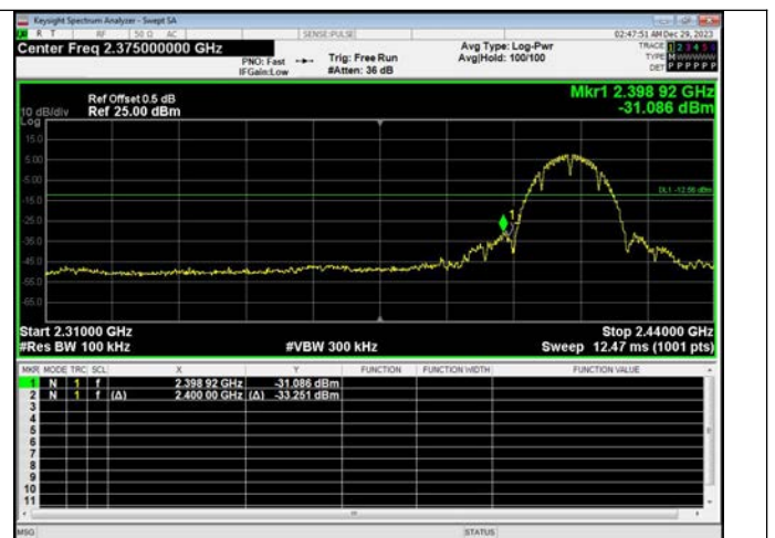
Out Of Band Emission IEEE 802.11b_Channel 1_20MHz_Antenna 1
