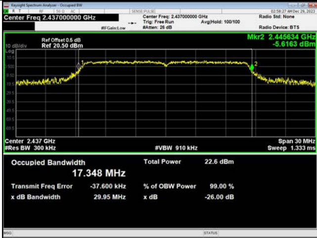
IEEE 802.11g_Channel 6_20MHz_Antenna 1
