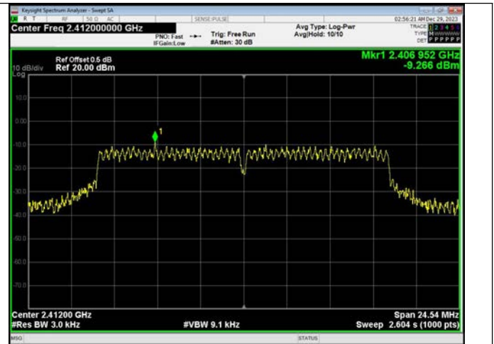
IEEE 802.11g_Channel 1_20MHz_Antenna 1
