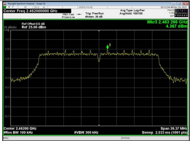
In-Band Reference Level IEEE 802.11n Channel 11 20MHz Antenna 1
