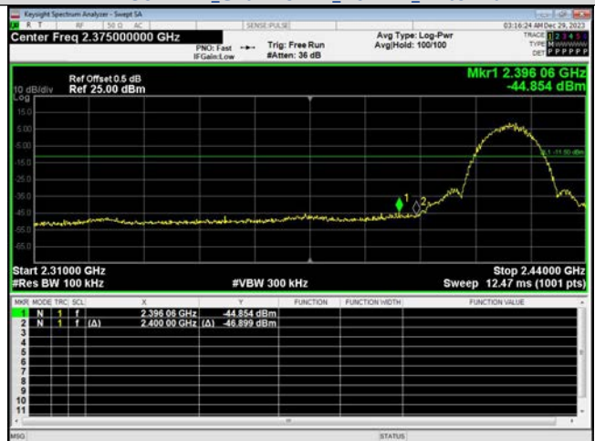
Out Of Band Emission IEEE 802.11n Channel 3 40MHz Antenna 1
