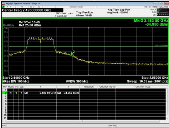
Out Of Band Emission IEEE 802.11n Channel 11 20MHz Antenna 1
