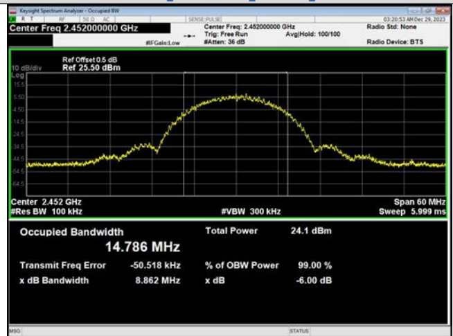
IEEE 802.11n_Channel 9_40MHz_Antenna 1
