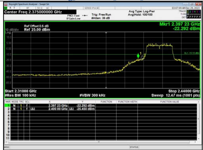
Out Of Band Emission IEEE 802.11n Channel 1_20MHz_Antenna 1
