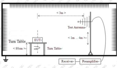
For radiated emissions from 30MHz to1GHz
