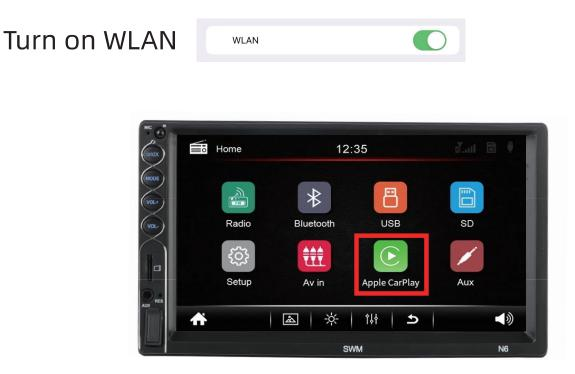
2.Turn on the Bluetooth of the iPhone, search for the Bluetooth Device naming "OKBox-BT\_\*\*\*\*" or "smartBox-\*\*\*\*" or "AIBox-BT\_\*\*\*\*" Pair it and allow the sync, finally click "Use CarPlay"
