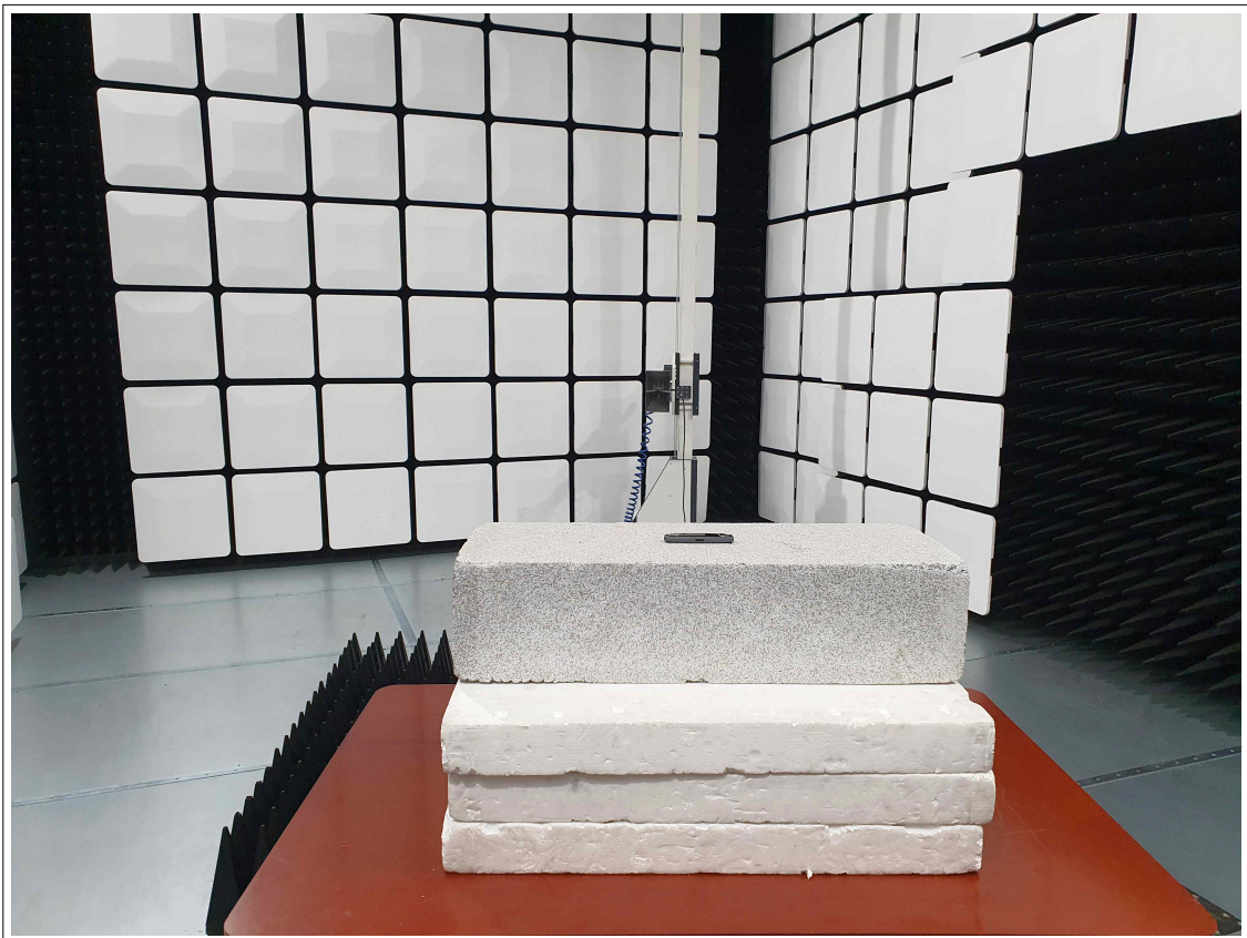
Radiated Emission Test Setup Above 1GHz_H
