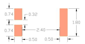
◆ 2<sup>nd</sup> Layout Dimensions in Clearance area(Size=8.0\*3.0mm)
