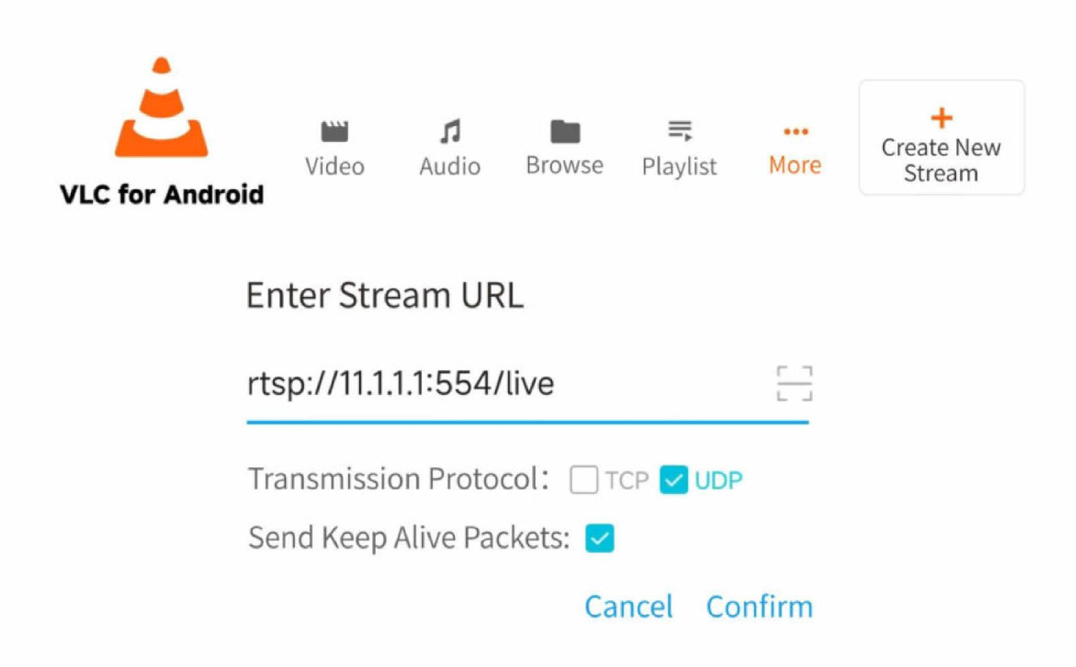
By entering the address and clicking "Connect", live stream the image feed on to your smartphone with the app of the device.
