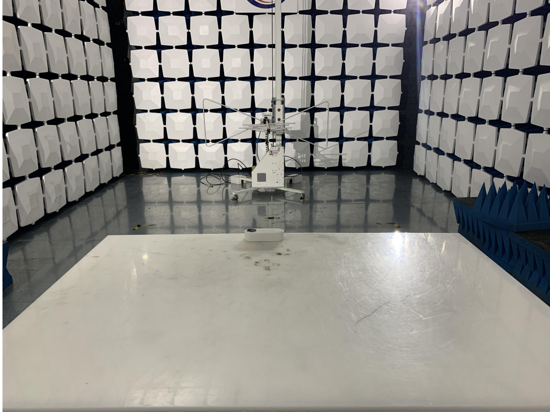
Above 1GHz for radiated emission test setup
