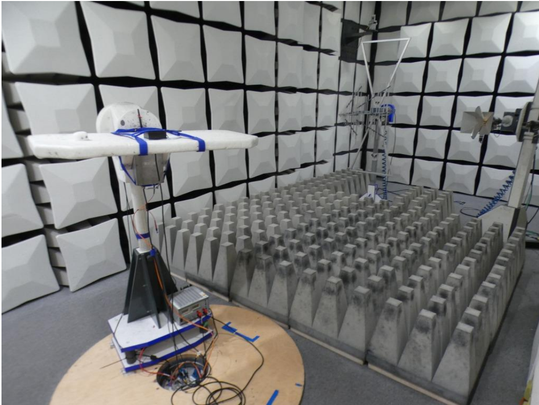
Photo 3: Test setup for radiated measurements, above 1 GHz
