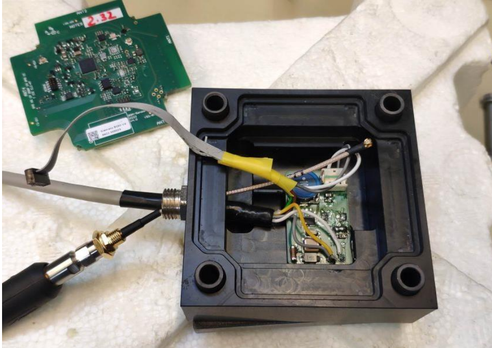
Figure 2: Supply module inside the housing
