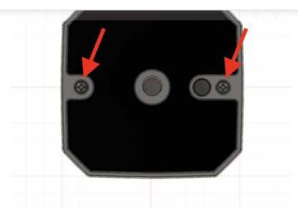
Remove the two screws that secure the baseplate. Do not lose the screws during removal.
