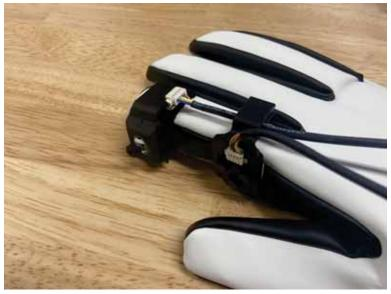
Secure the joystick with Velcro. It is also possible to fine-tune the mounting position.
