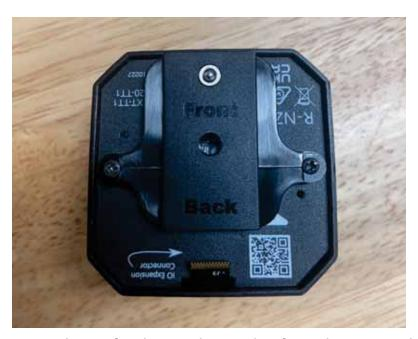
Remove the mounting adapter for the Tundra Tracker from the case and fix it to the tracker using the screws you removed earlier. There is a direction to install the adapter, so please install it in the same direction as the photo above.
