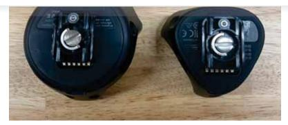
Remove the mounting adapter for Vive Tracker from the case and fix it using the included screws as shown in the image above.
