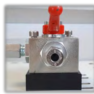
Holding the small plate using the hand tighten preliminary the three way valve, putting a spacer under it. Tighten it just to keep together all the parts allowing for horizontal movement of the valve.
