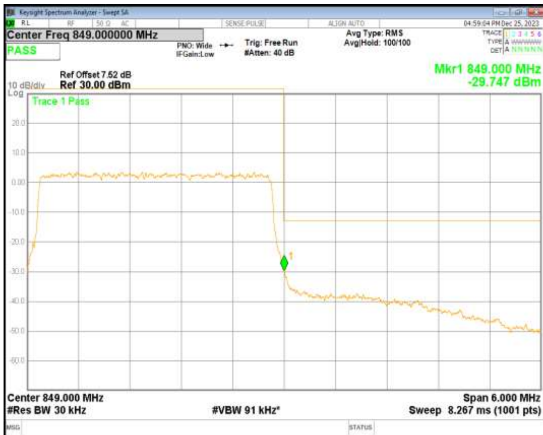
Band5 QPSK BW=5MHz Channel=20425 RB Size=25 Position=#0
