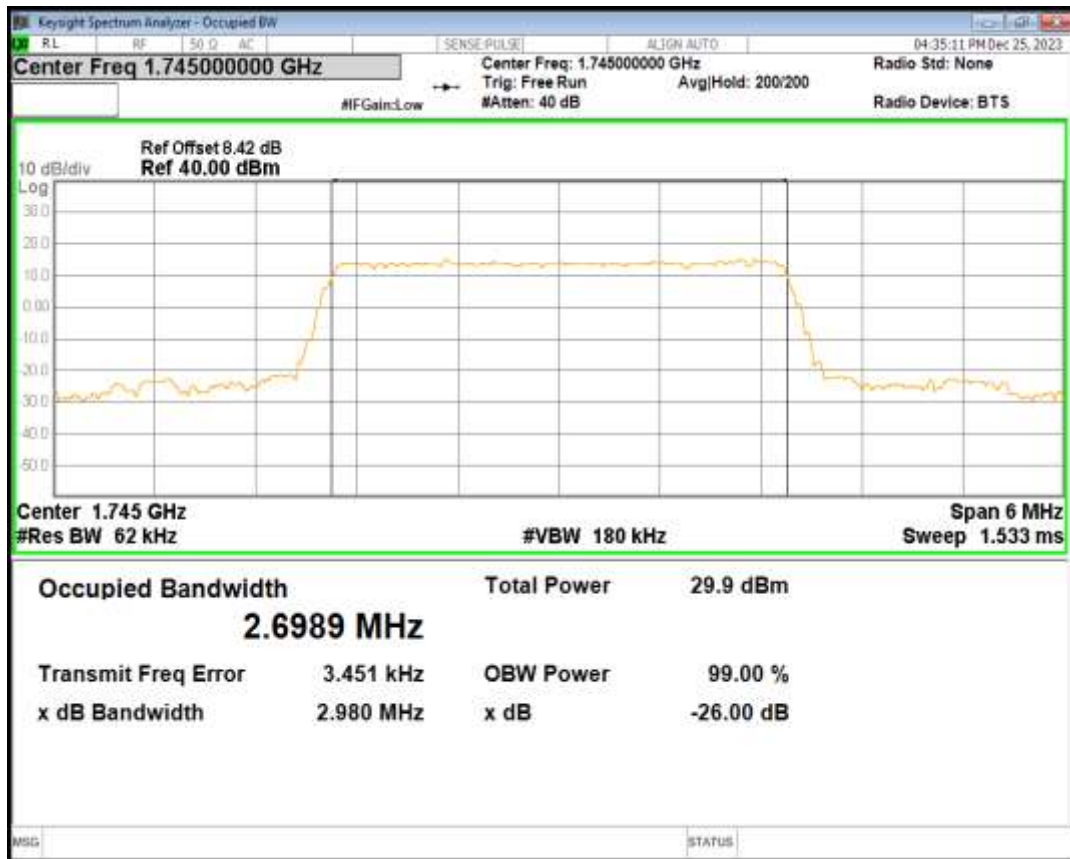
Band66 QPSK BW=3MHz Channel=132657 RB Size=15 Position=#0
